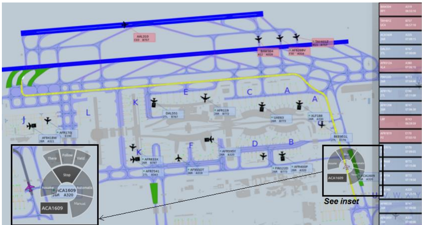
Figure 1: MoTa ground controller interface prototype, as in use for the South ground sector at CDG. The right panel is a list of all aircraft with information regarding their CTOT or arrival time and their flight status. The areas in green are potential holding points where the ATCO could send the aircraft. The physical location of the aircraft are represented by icons (those with a rectangle represent aircraft towed by an autonomous tug)
