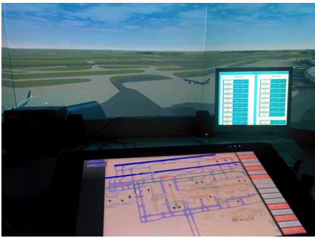
Figure 4: MoTa platform in the ATC simulator at ENAC, from the perspective of the user.
