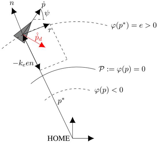
Figure 1: The direction to be followed by the UAV at the point  $p^*$  with respect to *HOME* for converging to  $\mathcal{P}$  is given by  $\hat{p}_d$ . The tangent and normal vectors  $\tau$  and  $n$  are calculated from  $\nabla\varphi(p^*)$ . The error distance  $e$  is calculated as  $\varphi(p^*)$ .
