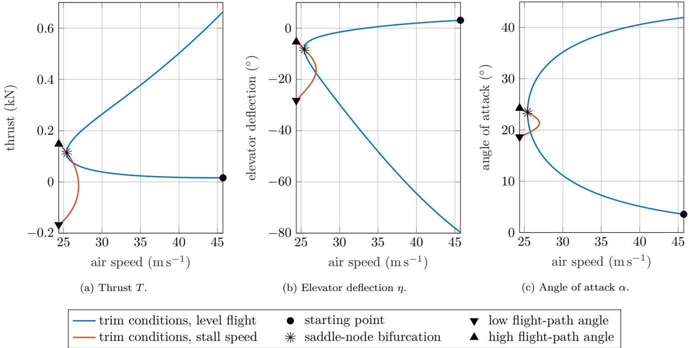
Fig. 1. Trim conditions obtained for level flight and varying speed, with respect to angle of attack, elevator deflection, and thrust. At stall speed, a saddle-node bifurcation occurs ( \* ) which depends on the respective flight-path angle ( — ).
