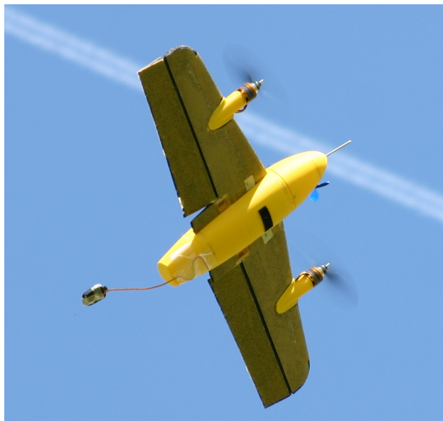
Figure 10. The development version of the Cyclone , in flight with a camera mounted on the rear.
