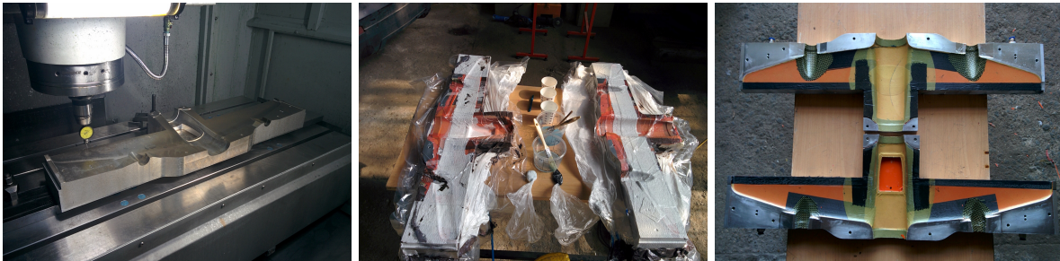
Figure 8. Manufacturing phases, CNC mold milling on the left, composite wet lay up vacuum bag in the middle, and finished skins on the right before closing the molds together.
