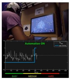
Fig. 1. It has been reported a real experience of how an EEG-based workload index (WEEG) can be used to trigger Adaptive Automation (AA) solutions embedded within an ATM simulator hosted at the Ecole Nationale de l'Aviation Civile (ENAC, Toulouse, France).
