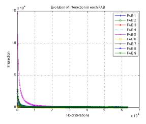
Fig. 17. Evolution of the interaction in each FAB for 26,122 trajectories during the optimization process using centralized ATFM model.
