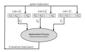
Fig. 5. FAB-Flight Interaction Matrix update process.
