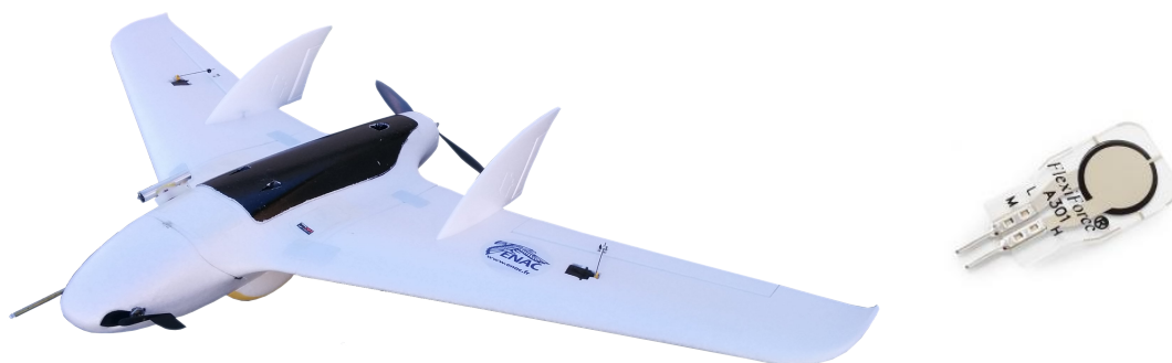
Figure 1. Mako aircraft general view on the left, and the FlexiForce A301 thin film force sensor on the right.
