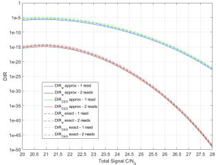
Figure 6 – DIR vs C/N<sub>0</sub> for GPS L1 C/A signal in AWGN channel conditions
