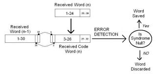
Figure 4 – GPS L1 C/A signal PC decoding process
