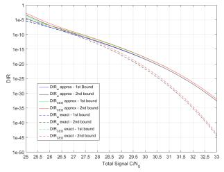
Figure 7 – DIR vs C/N<sub>0</sub> for GALILEO E1 OS signal in AWGN channel conditions
