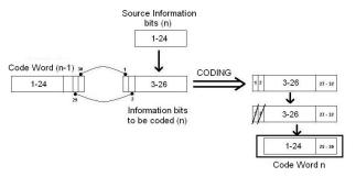
Figure 3 – GPS L1 C/A signal PC encoding process
