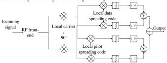
Fig. 10: Conceptual scheme of the data/pilot signal acquisition
