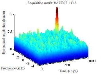
Fig. 2: Acquisition matrix output from serial search acquisition
