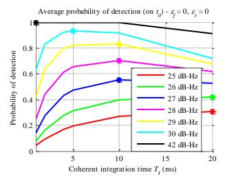
Fig. 8: Average probability of detection for different  $C/N_0$  values, for a dwell time of 20 ms
