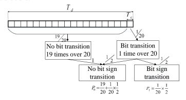
Fig. 7: Scheme to determine the probability of detection (GPS L1 C/A)
