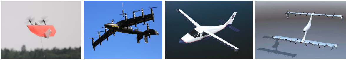
Figure 1. Tilt-Body micro air vehicle MAVION from ISAE, a small demonstrator of NASA’s GL-10 , the LEAPTech Program from JobyAviation, and the Pterosaur from ONERA.
