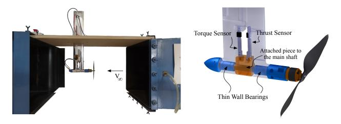
Figure 2. On the left, propulsion test bench mounted in the wind tunnel of ENAC, and on the right a detailed CAD view of the sensor integration and the moving parts is shown.
