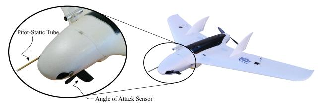
Figure 1. Integration of the pitot-static airspeed tube and the angle of attack sensor on the nose of the aircraft.
