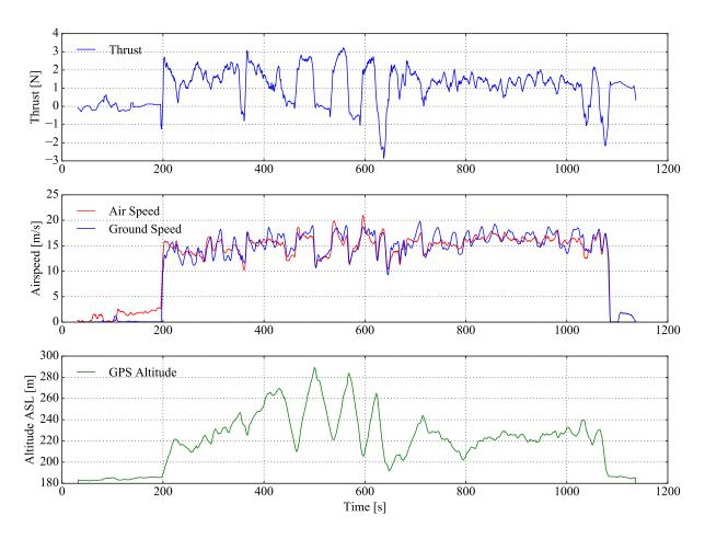
Figure 8. Preliminary flight results of the on-board thrust measurements are shown on the upper plot, with the airspeed and the ground speeds plotted in the middle, and finally the altitude information is shown on the bottom plot.
