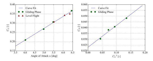
Figure 6. Lift coefficient versus angle of attack, and drag coefficient versus squared lift coefficient, estimated with the first method.
