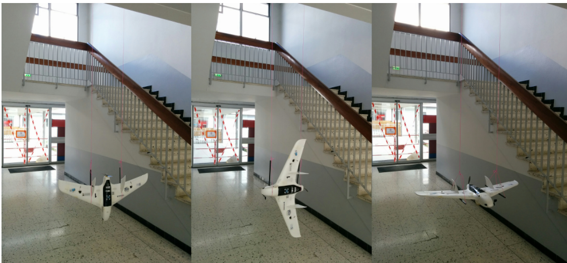
Figure 10. Moments of inertia measurements for each axis, I_{xx}, I_{yy}, I_{zz} .
