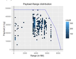
Figure 9. Payload-Range distribution
