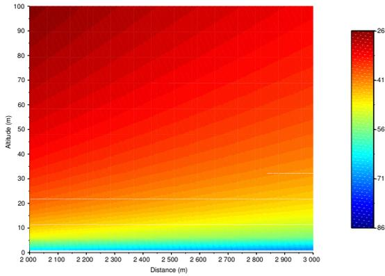
Fig. 2. Incident field (dBV/m) from a VOR station at 0 m in the absence of windturbines.
