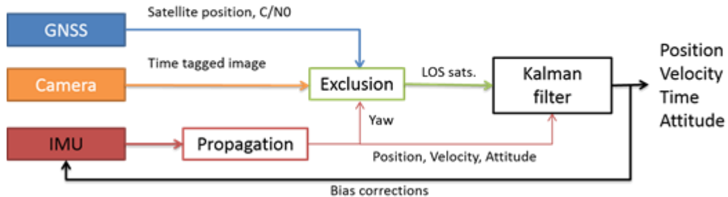
Figure 1: Integration scheme between GNSS, INS and camera exclusion
