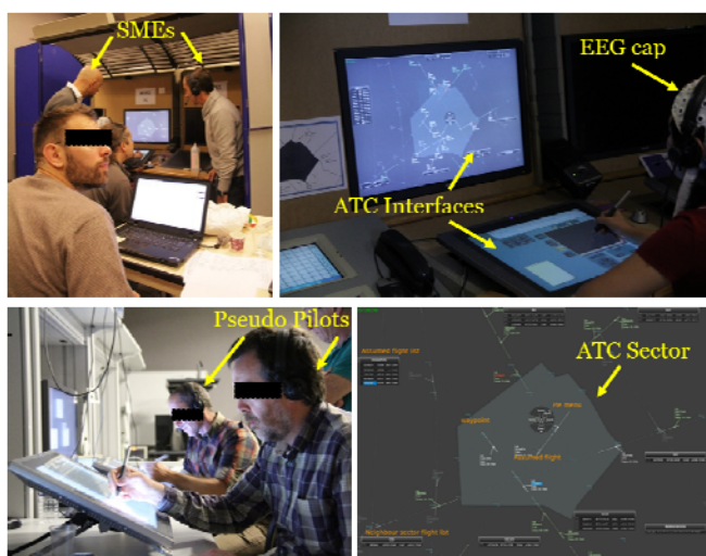
Figure 1. Experimental setup: prototypal ATCO working positions developed by ENAC (Toulouse, France) for a research simulator. The ATCO's brain activity has been recorded continuously and S, R and K events have been marked in order to recognize them within the entire EEG recording.
