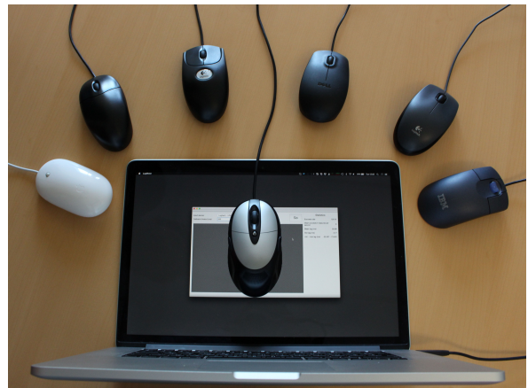
Figure 1: Sample setup used, with a Logitech MX310 mouse positioned on a horizontally-oriented laptop display. A particular texture is displayed and moved under the mouse sensor to fake displacements. Other mice discussed in the paper are positioned around the display.
