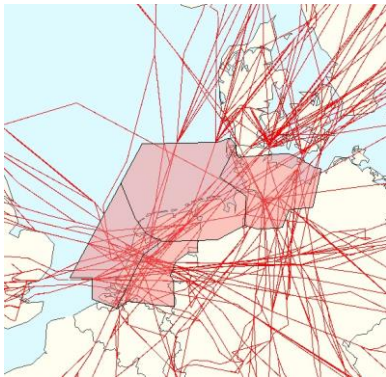
Figure 14. Planned trajectories in fixed-route network
