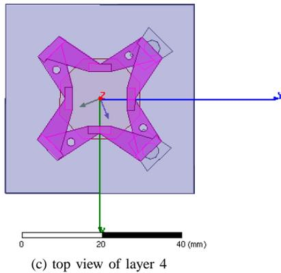
Fig. 9. Side and top views of the antenna.
