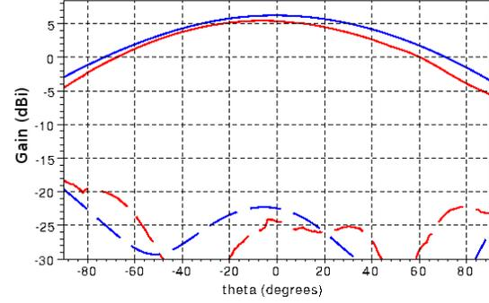
Fig. 13. Gain Pattern (dBi) in the  $xOz$  plane for  $\alpha_f = -j$ : RHCP measurement (red line), RHCP simulation (blue line), LHCP measurement (dashed red line), LHCP simulation (dashed blue line).
