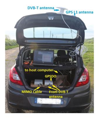
Fig. 6. USRP based test bench for outdoor testing
