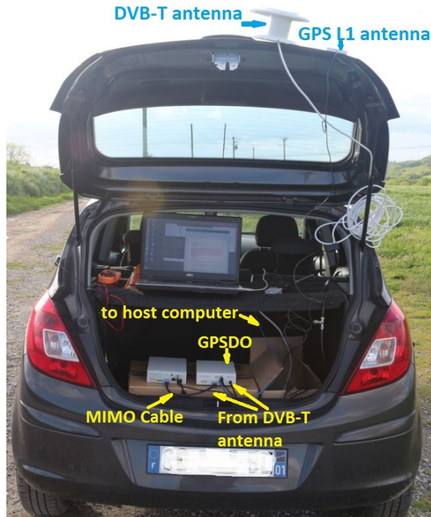
Fig. 6. USRP based test bench for outdoor testing
