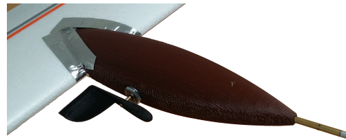
Fig. 4: Integration of the Pitot tube and the angle of attack sensor on the leading edge of the wing.
