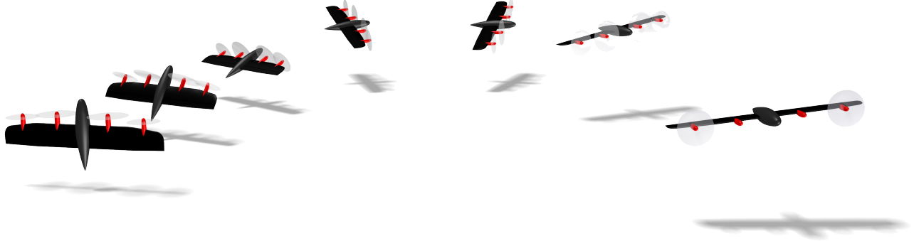
Fig. 2: Transitioning from four propeller stationary vertical take-off to two propeller high speed cruise phase.
