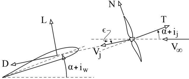
Fig. 4: Shows the wing incidence angle  $i_w$ , jet incidence angle  $i_j$ , angle of attack of the fuselage  $\alpha$  with the resultant lift  $L$ , drag  $D$ , thrust  $T$  and the propeller normal force  $N$ , propeller downwash  $\epsilon$ , jet slipstream  $V_j$ .
