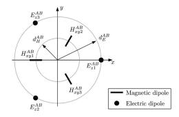
Fig. 3. Proposed topology of the dual-band vector sensor.
