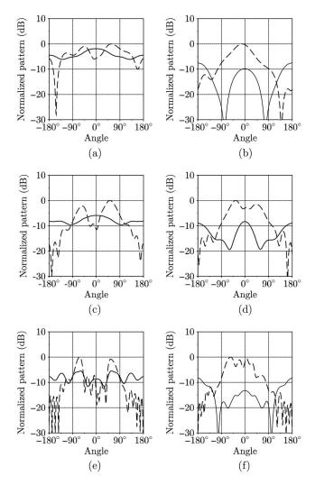
Fig. 18. Normalized patterns of (a)  $E_{z1}^C$  at 415 MHz; (b)  $H_{xy1}^C$  at 415 MHz; (c)  $E_{z1}^{AB}$  at 925 MHz; (d)  $H_{xy1}^{AB}$  at 925 MHz; (e)  $E_{z1}^{AB}$  at 1795 MHz; and (f)  $H_{xy1}^{AB}$  at 1795 MHz simulated in the E-plane (dashed line) and H-plane (solid line).
