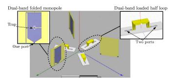
Fig. 5. Dual-band vector sensor using antennas spatially distributed and diversely polarized.
