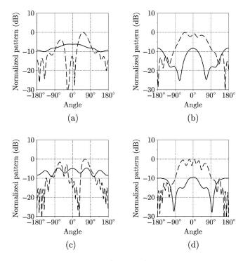
Fig. 7. Normalized patterns of  $E_{z1}^{AB}$  and  $H_{xy1}^{AB}$  in the E-plane (dashed line) and in the H-plane (solid line) (simulation results). (a)  $E_{z1}^{AB}$  at 925 MHz. (b)  $H_{xy1}^{AB}$  at 925 MHz. (c)  $E_{z1}^{AB}$  at 1795 MHz. (d)  $H_{xy1}^{AB}$  at 1795 MHz.
