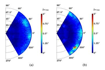
Fig. 12. Measured  $\Delta_{arms}(\phi,\theta)$  obtained with the dual-band vector sensor located on a  $800\times800~\mathrm{mm}$  metallic support at (a) 1000 and (b) 1800 MHz with  $P_r=-105~\mathrm{dBW~m^{-2}}$  (PNR =  $36~\mathrm{dB~m^{-2}}$ ), N=100, and L=20.
