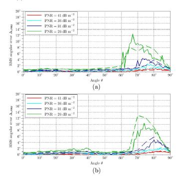
Fig. 14. Measured (dashed lines) and simulated (solid lines)  $\Delta_{arms}(\phi,\theta)$  according to  $\theta$  with (a)  $\phi$ =30° at 1000 MHz and (b)  $\phi$ =0° at 1800 MHZ for PNR = 41, 36, 31, and 26 dB  $m^{-2}$ ; N=100; and L = 20, in the worst case (azimuth angles of the maximum DoA error).
