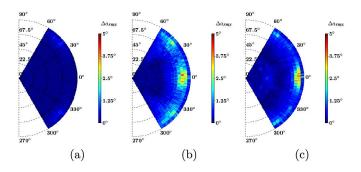
Fig. 19. Simulated  $\Delta_{arms}$  obtained with the tri-band vector sensor located on a  $800 \times 800$  mm metallic support: PNR = 36 dB m<sup>-2</sup>, N = 100, and L = 20. (a) 415; (b) 925; and (c) 1795 MHz
