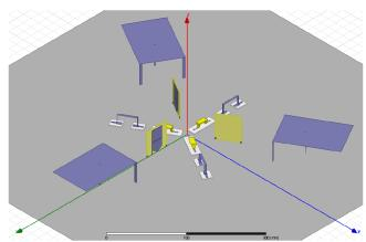
Fig. 16. Tri-band vector sensor using antennas spatially distributed and diversely polarized.
