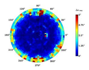
Fig. 2. Simulated  $\Delta_{arms}(\phi,\theta)$  at 2400 MHz as a function of  $\phi$  and  $\theta$  obtained with the initial vector sensor located on a  $800\times800$  mm metallic support with PNR =  $46~\mathrm{dB\,m^{-2}}$ , N=100, and L=20. The elevation angles  $\theta$  are given in the radial axis.
