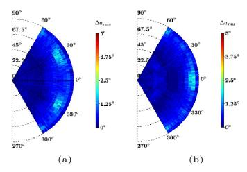
Fig. 8. Simulated  $\Delta_{arms}(\phi, \theta)$  obtained with the dual-band vector sensor located on a  $800 \times 800$  mm metallic support at (a) 1000 and (b) 1800 MHz with  $P_r = -105$  dBW m<sup>-2</sup> (PNR = 36 dB m<sup>-2</sup>), N=100, and L=20.
