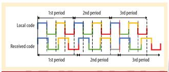
FIGURE 4 Code Doppler effect on the spreading code period
