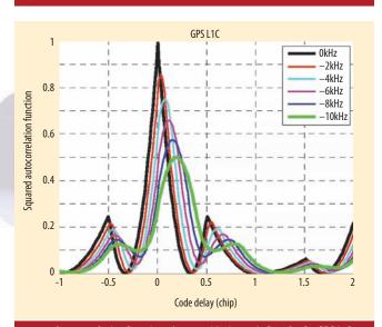
FIGURE 8 Autocorrelation function when considering code Doppler for GPS L1C on 50 ms  $\,$
