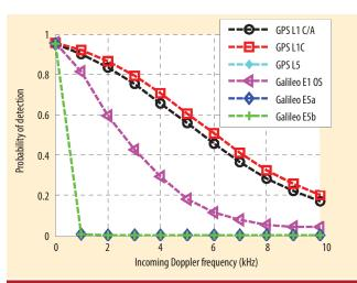
FIGURE 11 Probability of detection considering the total signal power and code Doppler
