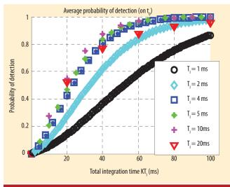
FIGURE 3 Average probability of detection at 27 dB-Hz for GPS L1 C/A
