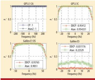
FIGURE 13 FLL schemes results when using total signal power
