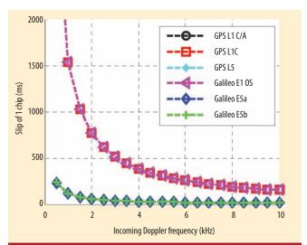
$\label{figure 9} \textbf{Figure 9 Time for the slip of one chip in function of the incoming Doppler frequency }$
