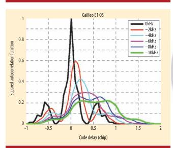
FIGURE 7 Autocorrelation function when considering code Doppler for Galileo E1 OS on 80 ms  $\,$
