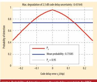
FIGURE 2 Probability of detection versus the code delay uncertainty for BPSK-modulated signals
