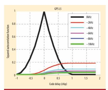
FIGURE 6 Autocorrelation function when considering code Doppler for GPS L5 on 217 ms
