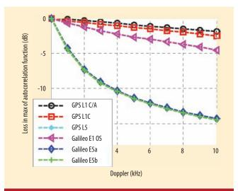
FIGURE 10 Losses on the autocorrelation function due to code Doppler
