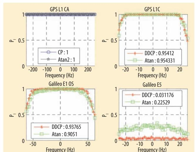
FIGURE 13 FLL schemes results when using total signal power
