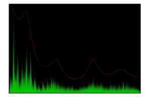
Figure 2: Linear predictive coding for a voice sample
