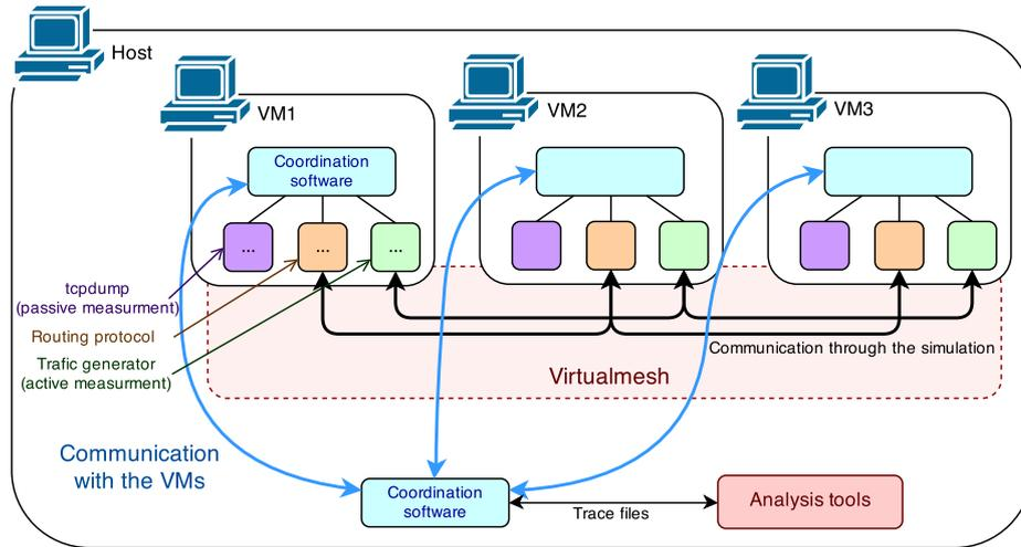
Figure 2: Testbed implementation
