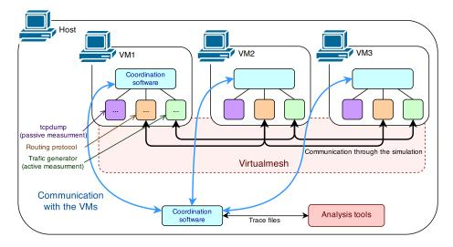
Fig. 1: Testbed implementation
