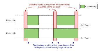
Fig. 4: "Unstable states" extracted from the measurement
