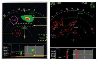
Figure 5: A) the current A380 ND, using a 2Dh+2Dv: the lower part (VSD: Vertical Situation Display) shows the vertical profile of the route; b) first prototype: we add a view of the RDT cells (in red) that intersect the "tilt" (upper, in blue), helping the pilot to select a cloud-free deviation.
