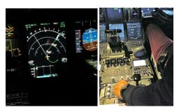
Figure 6: a) the actual A380 full-flight simulator navigation display and its "vertical cut" (white straight line); b) the pilot rotates the button to turn the vertical cut.
