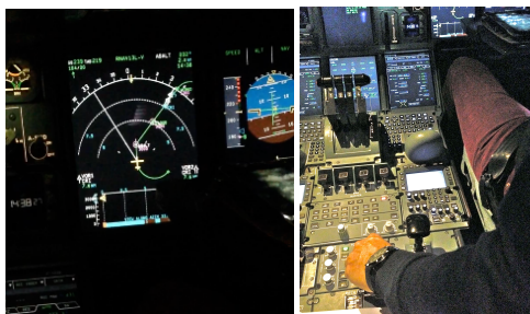
Figure 6: a) the actual A380 full-flight simulator navigation display and its “vertical cut” (white straight line); b) the pilot rotates the button to turn the vertical cut.
