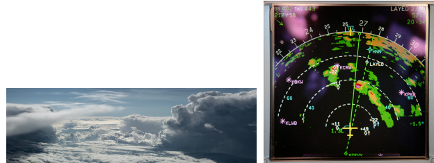
Figure 1: a) a panoramic view looking forward from the flight deck: dark clouds are towering thunderstorms. Thunderstorms are of course more dangerous in bad light conditions, during dark moonless nights; b) the navigation display of an airliner that shows the radar detection of the clouds on the left (red area indicates a definitely avoid cumulonimbus).
