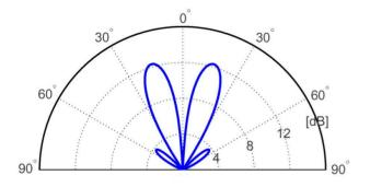
Fig. 5. Radiation pattern for a  $N_{\rm Tx}=12$  element array antenna and radius  $R_{\rm Tx}=\lambda$ . (From Mohammadi *et al* [9])
