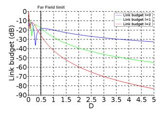
Fig. 6. Link budget as a function of the distance and the mode order 1.
