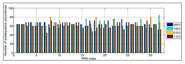
Figure 2 – number of 4-chip long subsequences ending by a rising transition in PRN 1 to 32. Each color corresponds to one subsequence.
