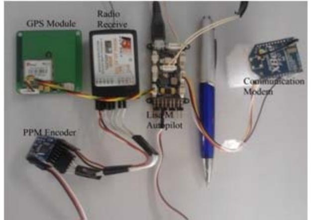
Figure 2 - Hardware Embedded in the Helicopter.
