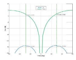
Fig. 4. Co and cross polarization at 0.76 GHz and  $\phi = 0$  deg.
