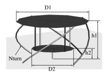
Fig. 1. Monopole antenna with quadrifilar cage (section II): h1=5.5cm, h2=1.5cm, D1=12cm, D2=7cm, Wire diameter 2mm,  $Nturn=\frac{25}{25}$
