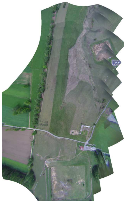
Figure 12: The result of the projection of ten images on the 3D map.
