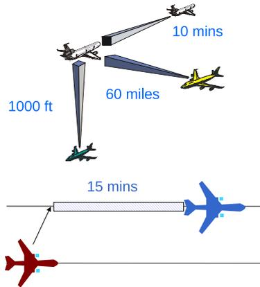
Figure 2: Oceanic Separation Standard
