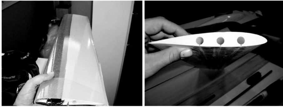
Figure 10. Surface quality and holes for steel rods simulating battery weight and inertia.
