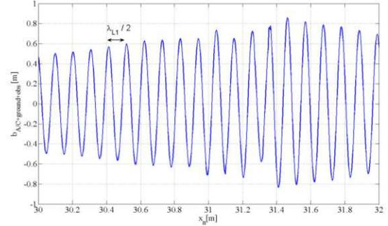
Figure 5: Evolution of  $b_{A/C+ground+obs}$  along a portion of [AB] – elevation angle =  $35^\circ$ , azimuth angle =  $0^\circ$ , illuminated façade parallel to the Y axis, aircraft centerline parallel to the X axis and points in the North direction
