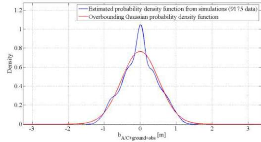
**Figure 6: PDF of the estimated distribution of  $b_{A/C+ground+obs}$  from simulations in the impact zone of a 10m metallic cube, elevation angle = 35°, azimuth angle = 0°, illuminated façade parallel to the Y axis, aircraft centerline parallel to the X axis, and PDF of the over-bounding Gaussian distribution**
