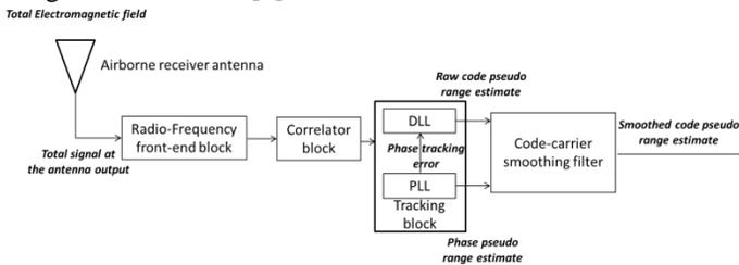
Figure 1: signal processing blocks of a GNSS receiver
