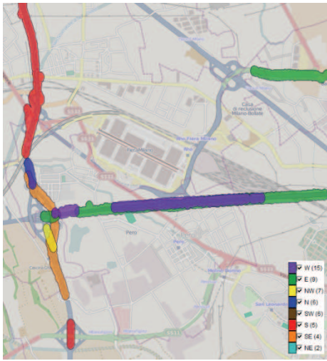
Figure 4. A map fragment shows the spatial buffers enclosing SD-clusters of low speed events.
