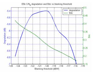
Figure 19 Simulated E5b C/N<sub>0</sub> degradation and Bdc versus blanking threshold over the European hot-spot
