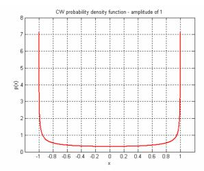
Figure 13 Unity-amplitude sinusoidal signal probability density function.
