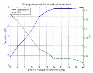
Figure 21 Theoretical E5b C/N<sub>0</sub> degradation and Bdc as a function of the bilateral reallocation bandwidth over the European hot-spot
