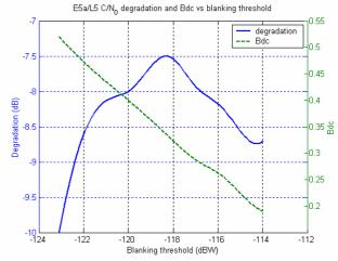
Figure 18 Simulated E5a/L5 C/N<sub>0</sub> degradation and Bdc versus blanking threshold over the European hot-spot
