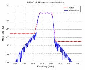
Figure 3 EUROCAE interference masks and simulated filter on E5b
