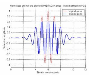
Figure 11 Original DME/TACAN pulse and the blanked version
