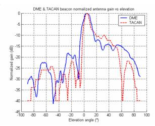
Figure 14 Considered DME/TACAN beacon antenna gains versus elevation
