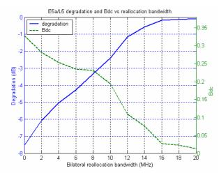
Figure 20 Theoretical E5a/L5 C/N<sub>0</sub> degradation and Bdc as a function of the bilateral reallocation bandwidth over the European hot-spot
