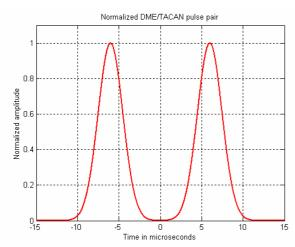
Figure 4 Normalized DME/TACAN pulse pair
