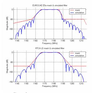
Figure 2 RTCA and EUROCAE interference masks and simulated filters on E5a/L5 bands
