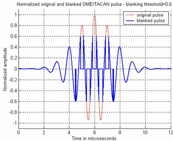
Figure 11 Original DME/TACAN pulse and the blanked version
