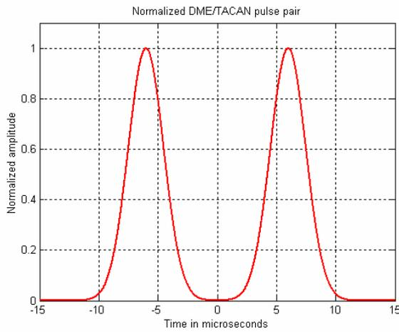
Figure 4 Normalized DME/TACAN pulse pair
