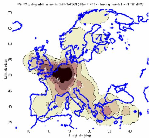
Figure 17 Theoretical E5b degradation over Europe due to DME/TACAN signals – blanking threshold -120.0 dBW
