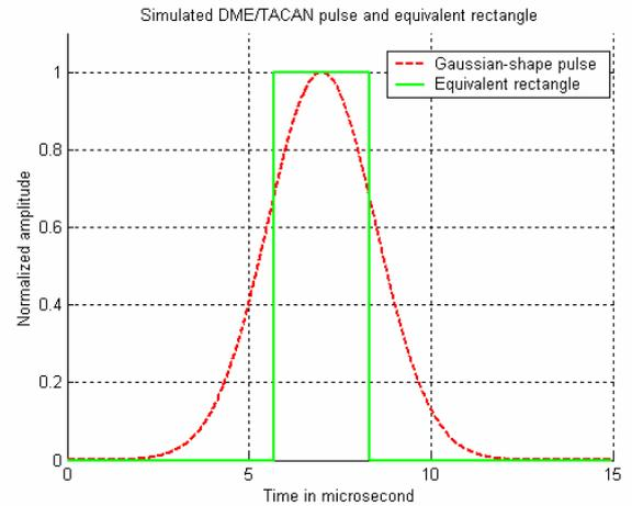
Figure 7 Simulated DME/TACAN pulse and equivalent rectangle
