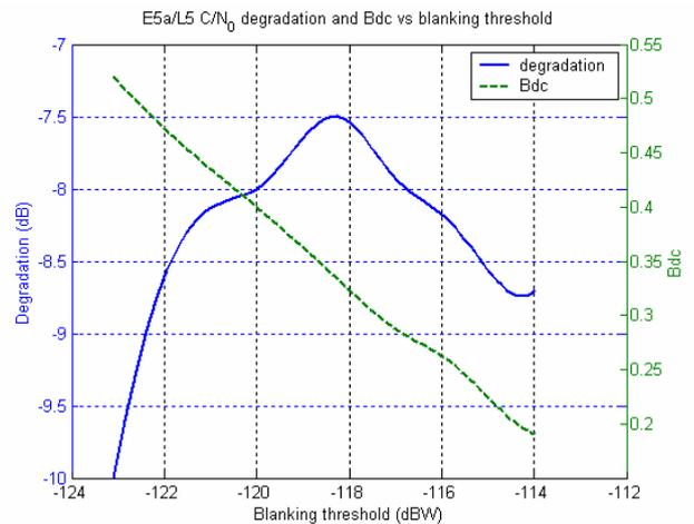
Figure 18 Simulated E5a/L5  $C/N_0$  degradation and Bdc versus blanking threshold over the European hot-spot
