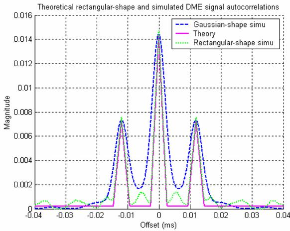
Figure 8 Gaussian-shape and rectangular-shape simulated and theoretical DME signal autocorrelation
