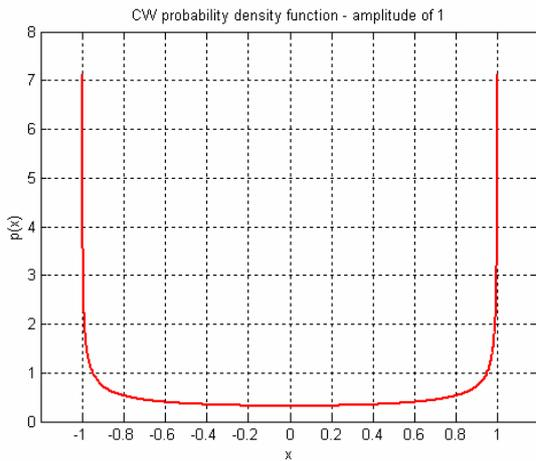
Figure 13 Unity-amplitude sinusoidal signal probability density function.
