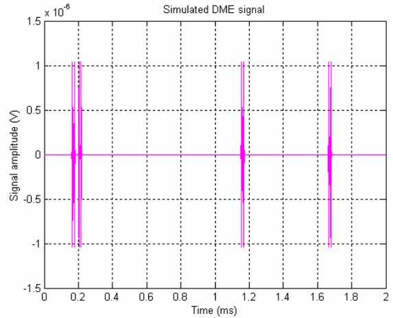
Figure 5 Simulated DME signal over 2 ms
