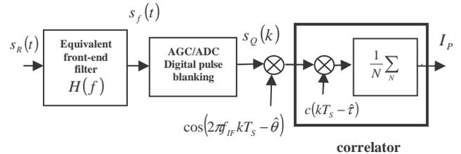
Figure 1 Single channel receiver front-end and correlator
