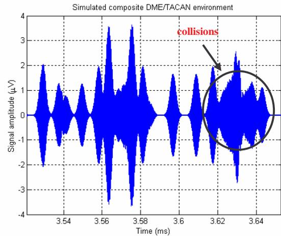
Figure 6 Example of composite DME/TACAN signals environment
