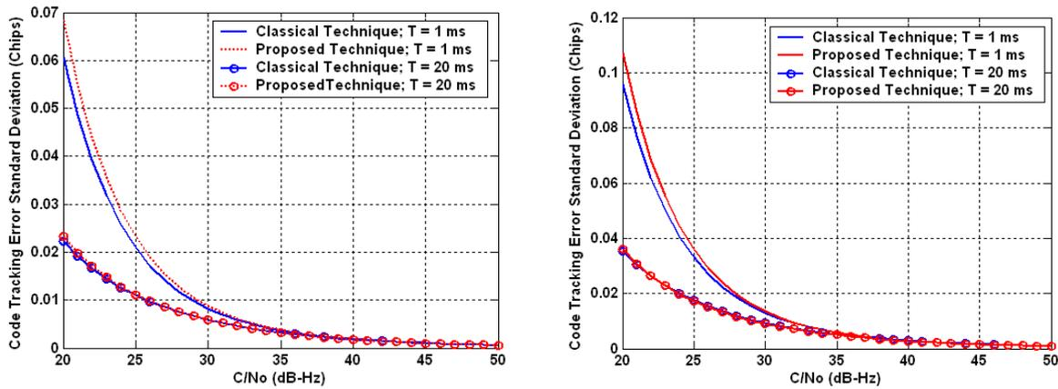
Fig. 4 – Comparison of the Theoretical Traditional and Proposed BOC(n,n) Code Tracking Error Standard Deviation for  $B_L = 1$  Hz, an Early-Late Spacing of 0.2 (Left) and 0.5 (Right) Chips and an Integration Time of 1 and 20 ms
