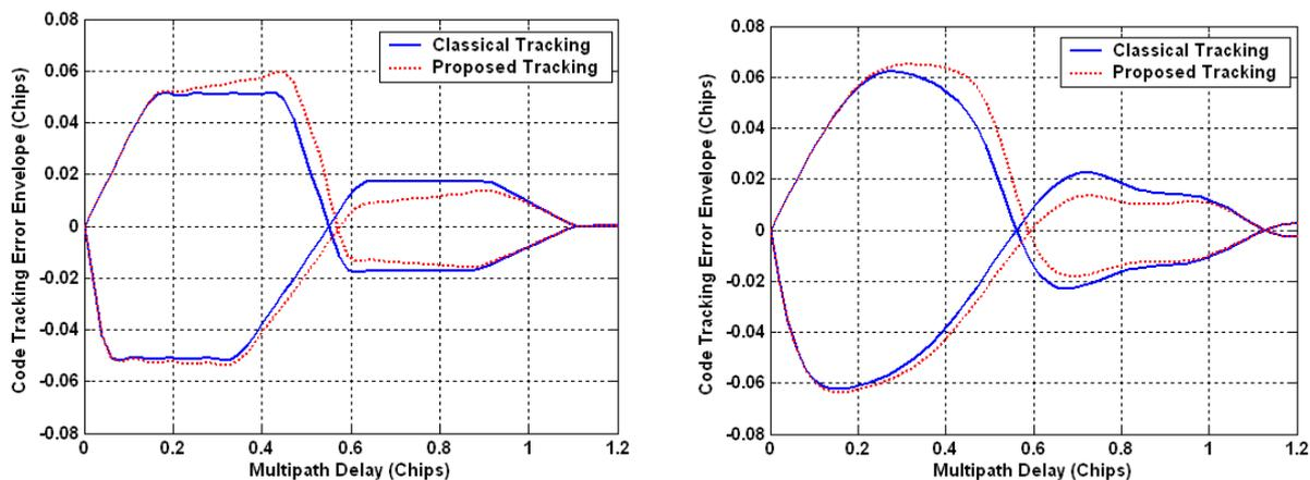
Fig. 5 – Multipath Envelope of the Classical and Proposed BOC(1,1) Tracking Techniques for a Signal-to-Multipath-Power-Ratio of 3 dB,  $d = 0.205$  Chips and a Double Sided Front-End Filter of 24 MHz (Left) and 6 MHz (Right)
