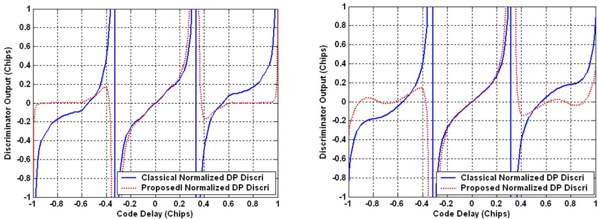
Fig. 2 – Normalized Discriminator Output for BOC(1,1) Classical and Proposed Dot-Product Discriminators for a Double-Sided Front-End Filter Bandwidth of 24 (Left) and 6 (Right) MHz and  $d = 0.205$  Chips
