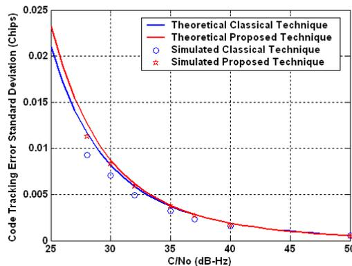
Fig. 7 – Simulation Results for the Code Tracking Error Standard Deviation in Thermal Noise Only for Traditional and Proposed BOC(n,n) Tracking Techniques for  $d = 0.2$  Chips
