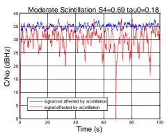
Figure 7 Impact of scintillation on received signal power
