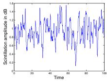
Figure 1 Scintillation amplitude for the weak scintillation scenario with S4=0.51 and τ0=0.71
