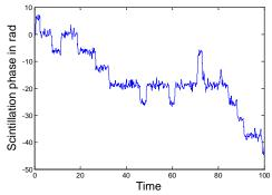
Figure 6 Scintillation phase for the severe scintillation scenario with S4=0.87 and τ0=0.18
