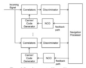
Figure 9 Generic vector tracking architecture
