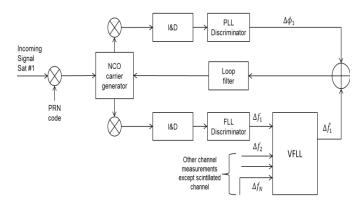
Figure 10 Implemented VFLL-assisted PLL architecture
