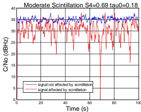
**Figure 7 Impact of scintillation on received signal power**
