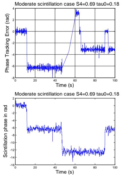
**Figure 8 Impact of scintillation on signal phase**
