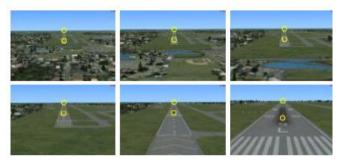
Figure 4 – Set of reference frames taken from a video as the UAV gets closer to the runway. The vanishing point and a point at the beginning of the runway (the spot where the UAV should touch down) are annotated in each frame. [15]
