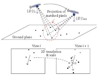
Figure 10 – Principle of trajectory recovery [19]
