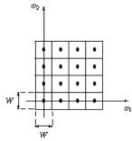
Figure 8 – Sub-grid decomposition [18]
