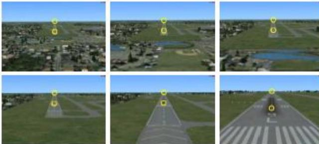
**Figure 4 – Set of reference frames taken from a video as the UAV gets closer to the runway. The vanishing point and a point at the beginning of the runway (the spot where the UAV should touch down) are annotated in each frame. [15]**
