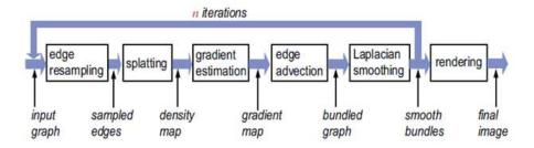
Figure 7. Pipeline to obtain a bundled graph.
