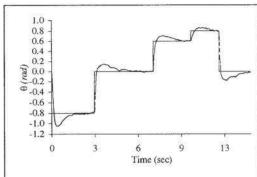
**Figure 4.** Response of Inverted pendulum system using ANT control,  $|\theta_d| \le 0.8$  radian.
