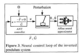
Figure 3 shows the ANT control structure of the inverted pendulum system, where
