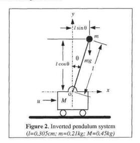
Taking the notations as shown in the above figure and assuming that the pendulum mass is concentrated at the end of a massless rode, the following mathematical model of the system is obtained [3].
